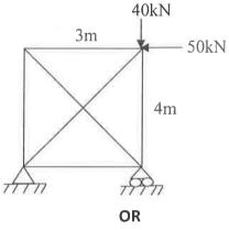
Q.2(B) Determine the forces in all the members of a truss shown in Figure. Take areas as 2000mm² for vertical and horizontal, and 3000mm² for diagonal members.
